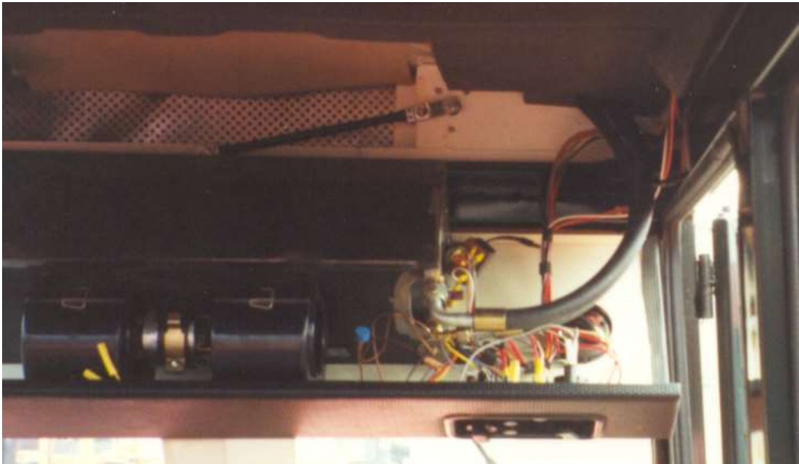
Heat/cool box showing refrigerant hose routing.
