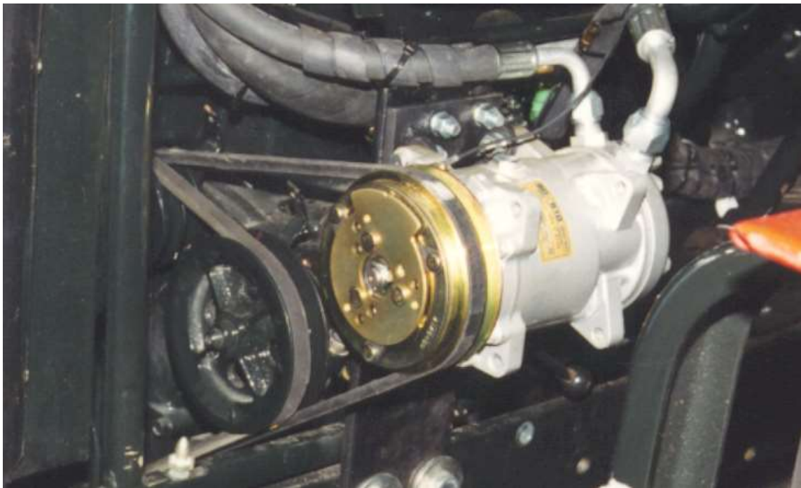
Compressor mounted in position.
